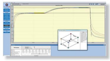
A separate software package, "Thermal View Survey" is available for surveying furnaces to AMS2750 requirements. Featuring thermocouple and data logger correction factors, user defined TUS levels and tolerances, View Frame analysis, overshoot search, data import / export, printed AMS2750 report. Contact us for a demo version!
