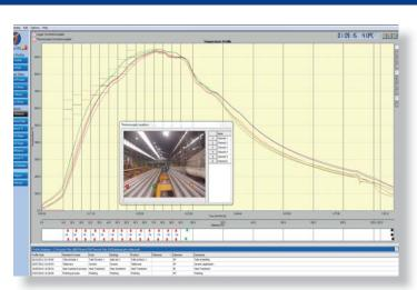
The temperature profile is displayed in the graphics window of the Thermal View software. Thermocouple profiles can be switched on or off individually and you can zoom in for more detailed analysis.
