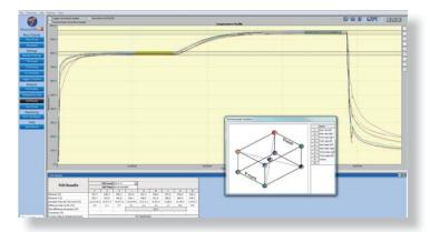
A seperate software package, "Thermal View Survey" is avaliable for surveying furnaces to industry requirements. Featuring thermocouple and data logger correction factors, user defined TUS leves and tolerances, View Frame anaylsis, over shoot search, data import / export, printed report. Contact us for a demo version!
